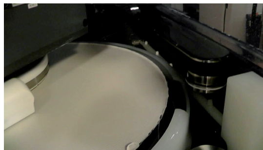
Photo A: Sweeping over the pad edge when using a suede-type soft pad may tear the pad edge.
